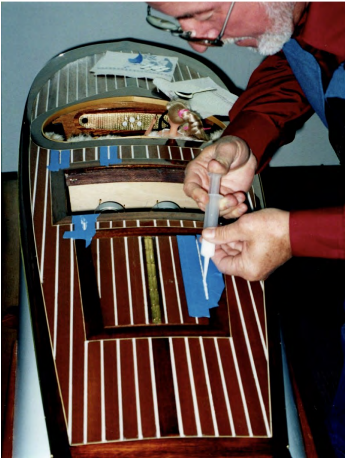
The seams between the deck boards were filled with a silicone tub caulking. Prior to caulking, Captain Rogers inserted a cord to help fill the void and to facilitate the removal of caulking in case he was dissatisfied with any of the seams.
