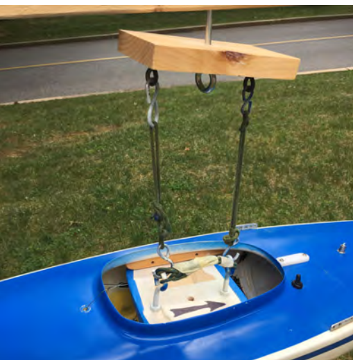
The "Key" inserted and positioned to support the suspended hull.
